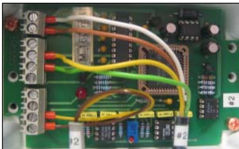
Figure 23: Connecting the Pyrradiometer cable to CONSH1 #2
