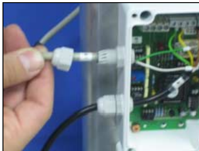
Figure 24: Connecting the Pyrradiometer cable to CONSH1 #1
