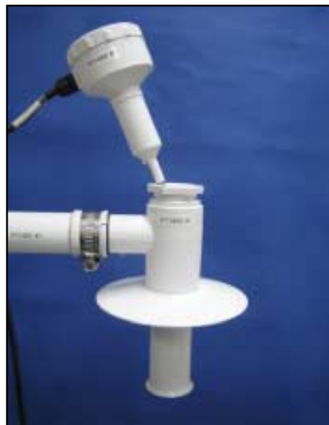
Figure 20: Mounting the upper temperature sensor PT 1000 #1
