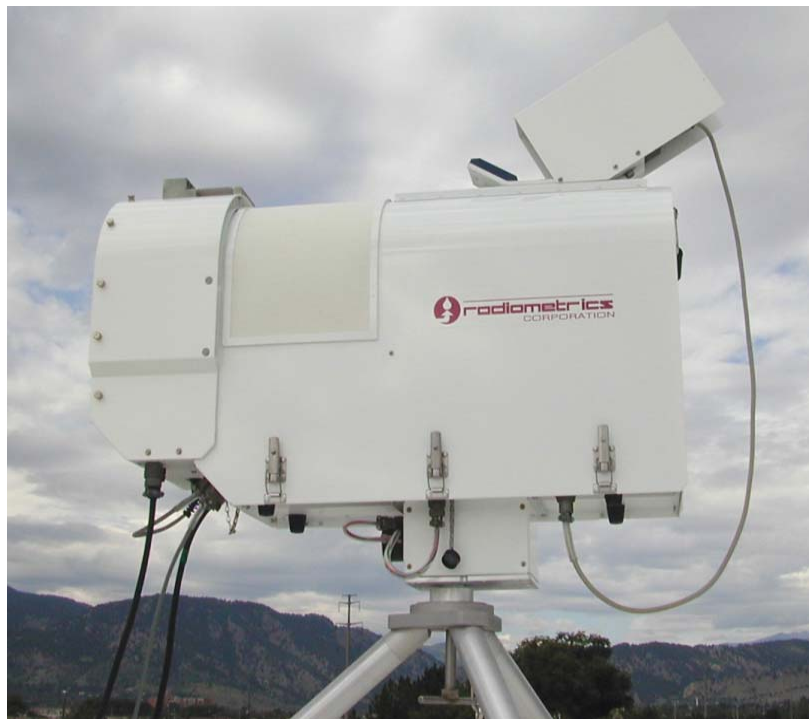
Figure 1. Radiometrics TP/WVP-3000 temperature, humidity and cloud liquid profiling radiometer.
